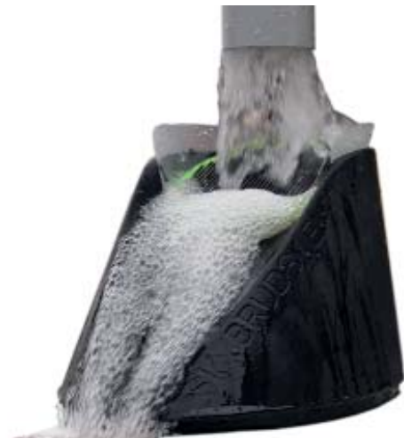
LAP - Grøn By - Skybrudsventil, test. VandVender.
